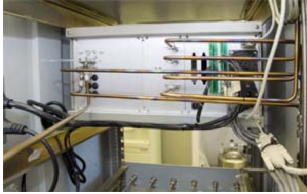
Gas samples enter the BevAlert analyzer via rear tubing. Unit transmits continuous data to Praxair.
