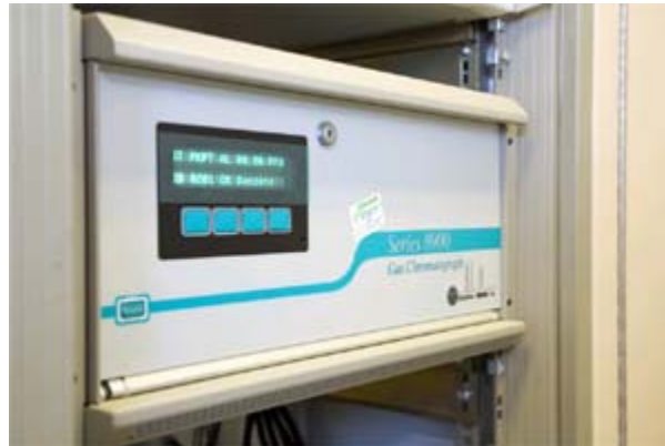
BevAlert's digital display provides easy-to-read status of sample.
